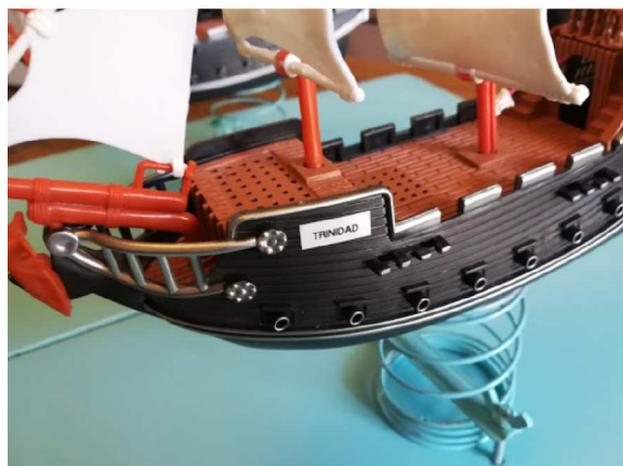
**Figure 2:** Model of the 3D printed caravel mounted on a spring and wooden plate (simulating the movement of the caravel in the sea).
